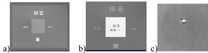
Fig. 3. a) Image of IR target generated by thermal imager, b) Image of VIS target generated by CCD camera, c) Image of laser target irradiated by LRF and seen by a thermal imager
