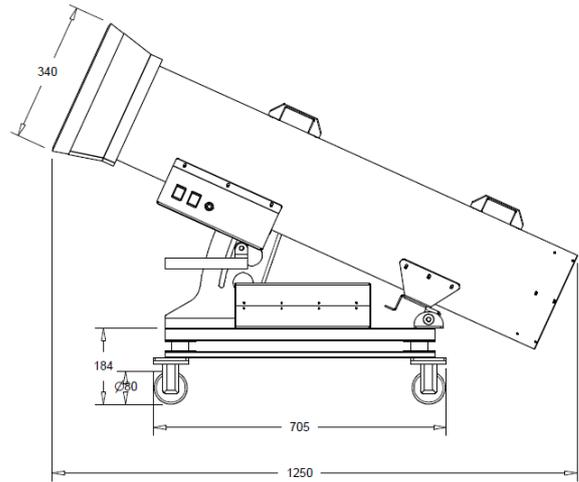
Fig. 2. 2D drawing of JAT200 boresight station
