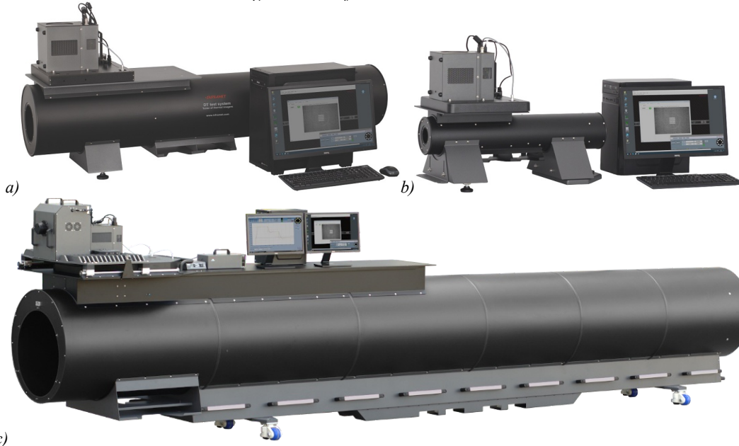
Fig. 2. Photos of three test systems built using three collimators (long black tubes) of different aperture and focal length.
