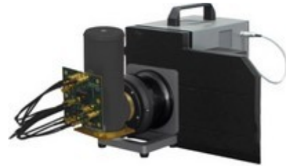
Fig. 2. FAPA-N system for response/noise tests of IR FPAs/camera cores
