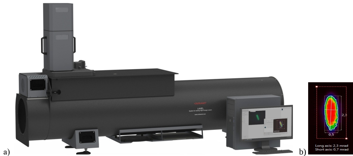
Fig. 1. LAHEL240 test system: a)photo, b)angular spatial intensity distribution of tested HEL
