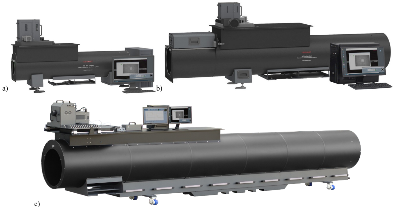
Fig. 1. Photo of several versions of MS3 test system different aperture and test capabilities: a) MS5120, b) MS30200 c) MS60600
