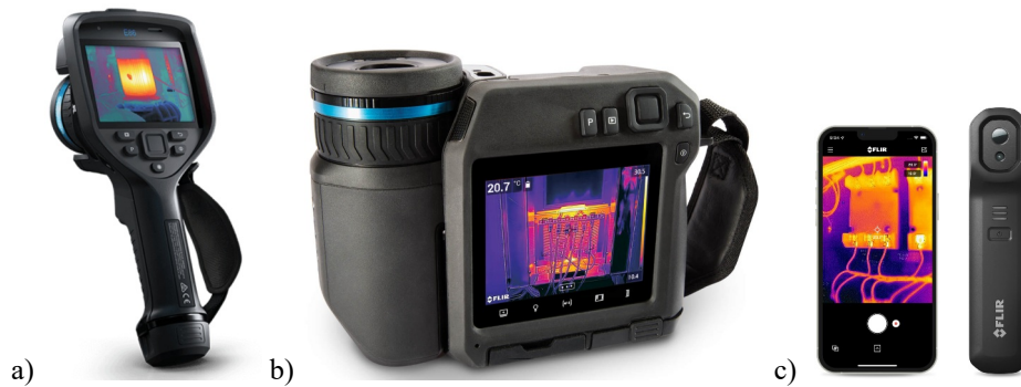
Fig. 32. Three forms of handheld cameras: a) handheld frame camera (FLIR E86 24°) b)photo like camera (FLIR T560 24°), c) smartphone attachment camera (FLIR ONE® Edge Pro),
