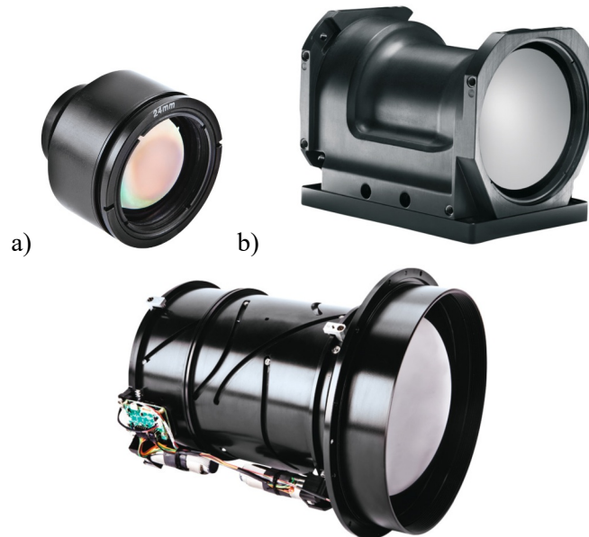
Fig. 15. Photos of exemplary IR objectives representing three main groups: a) 1-FOV objective (Ophir SupIR 24 mm f/1.0), b) M-FOV (Ophir SupIR 45/135 mm, f/1.1, f/1.6 Motorized Focus LWIR XGA), c) zoom objective (Ophir SupIR 40-300 mm f/1.5 LWIR Motorized Continuous Zoom SXGA Imaging Lenses)
