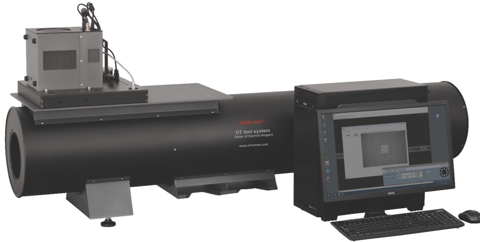
Fig. 41. Exemplary system (DT150 from INFRAMET[116] ) for testing thermal imagers composed from six main blocks: off axis reflective collimator, area blackbody, set of targets, PC, frame grabber, software
